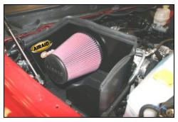
**15.** Install the Airaid Premium Filter (#1) onto the tube on the CAD and tighten the hose clamp. Next install the weather strip (#5) on the top of the CAD as shown. Apply the Airaid Foil Decal onto the Panel as shown.
