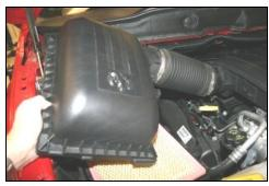
**2.** Unlatch 4 clips on the factory airbox lid and remove the lid and intake hose assembly. Remove the factory air filter.
