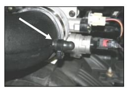
**14.** Install the provided rubber cap (#11), and speed clamp (#8) onto the nipple on the Modular Intake Tube (#3).
