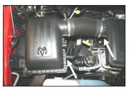
1. **Disconnect the negative battery cable!** Loosen the hose clamp on the resonator. Disconnect the breather hose going into the factory airbox lid.
